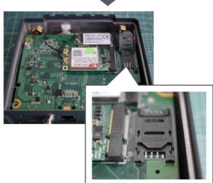
2 Lift up the SIM card slot (1) and insert the SIM card (2).
