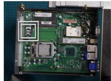
Be sure not to remove the yellow object attached to the site where the heat sink was removed. This is the heat sink pad, which allows heat to escape from the device via the heat sink. Moreover, heat sink thermal paste is applied to the CPU portion. Please do not remove this paste. If there is insufficient thermal paste, additional store-bought thermal paste may be added.
